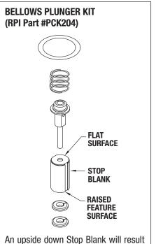
an upside down Stop Blank will result in a P2 Error Code. Make sure the flat surface is up and the raised feature surface is down.
